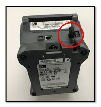
• Using a Philips-Head #2 screwdriver, remove the three screws that attach the power supply assembly to the bottom of the printer and then pull the power supply away from the printer.
